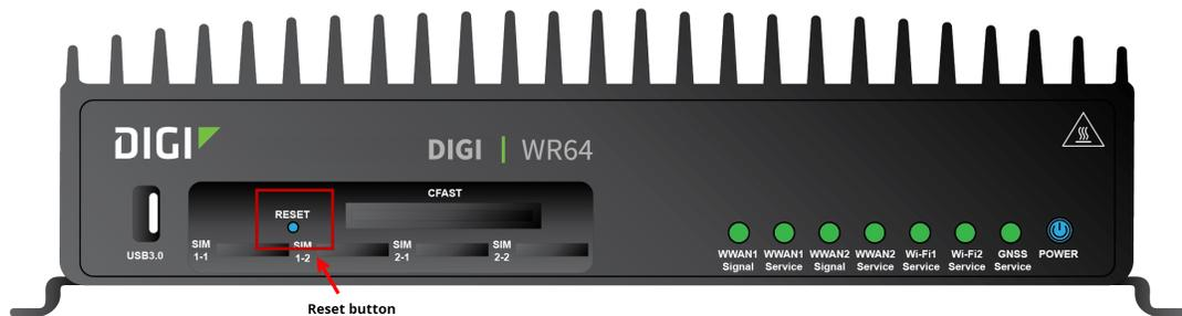
2. Press and hold the **Reset** button for **15** seconds. The device reboots automatically. The device resets to factory defaults. Follow the instructions in the [Quick start](#) to reconfigure the device.
