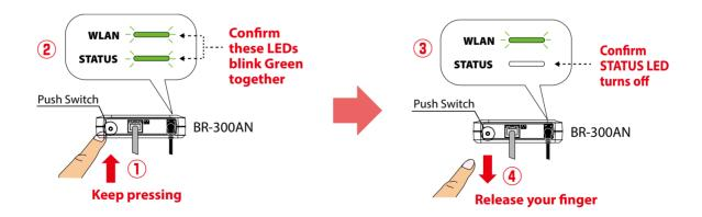
**6.** The BR-300AN and the Access Point will start to communicate each other. When the configuration finished successfully, the WLAN LED turns Green and the STATUS LED turns or blinks Green.
