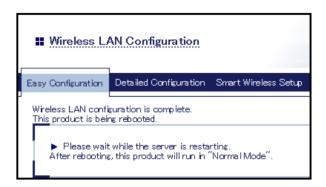
When you wish to bridge the PC used for this configuration wirelessly, restart the PC. To bridge another device wirelessly, turn off both BR-300AN and PC, remove the BR-300AN from the PC and connect the BR-300AN to the device you wish to use wirelessly using a network cable. For details, refer to **Connecting Non-wireless Devices** in the next page.
