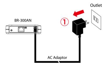
**2.** Press and hold the push switch on the front while inserting the AC adaptor back into the electrical outlet.
