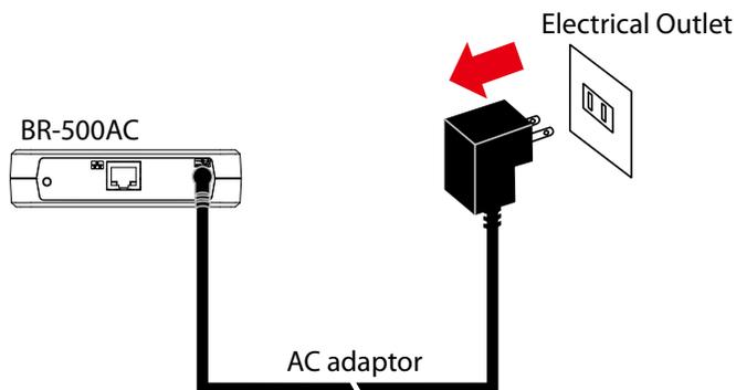
2. Press and hold the push switch on the front while inserting the AC adaptor back into the electrical outlet.
